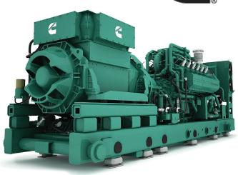
Alternator – Several alternator sizes offer selectable voltage and temperature rise with low reactance 2/3 pitch windings; low waveform distortion with non-linear loads, fault clearing shortcircuit capability, class F or H insulation (see Alternator Data Sheet for details), bearing and stator RTDs and anti-condensation heater. Mechanically strengthened for use on utility paralleling with unreliable grid.
